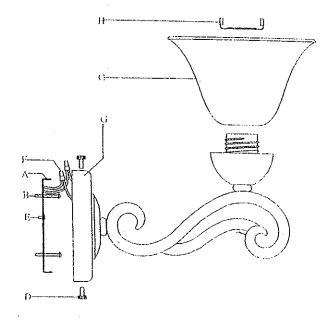
NOTE: THIS FIXTURE IS RATED FOR A 100-WATT STANDARD BULB (NOT INCLUDED). TO PREVENT THE RISK OF FIRE. DO NOT EXCEED RECOMMENDED WATTAGE.
